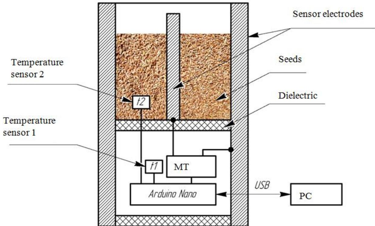
Figure 1: General view of the USB moisture meter
