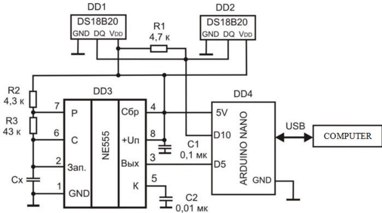
Figure 2: Schematic diagram of the USB moisture meter
